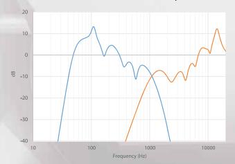
In conventional PA loudspeakers, compression drivers are paired with direct radiating cone drivers, crossed over at 1-2 kHz. The low crossover point creates distortion in the compression driver. Furthermore substantial equalisation is used to obtain a flat response, reducing headroom.
