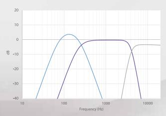
The Funktion-One approach is to use a dedicated wide bandwidth midrange. This reduces distortion and improves audio quality by moving crossover points outside the vocal range, allowing optimised mid-bass driver parameters and high frequency drivers to be transparent.
