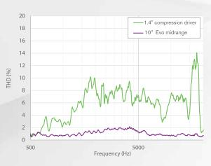
Compression drivers can produce as much as 10% THD in the midrange. Comparatively, the THD of the Evo 10" is substantially less than 2% throughout most of its range.
