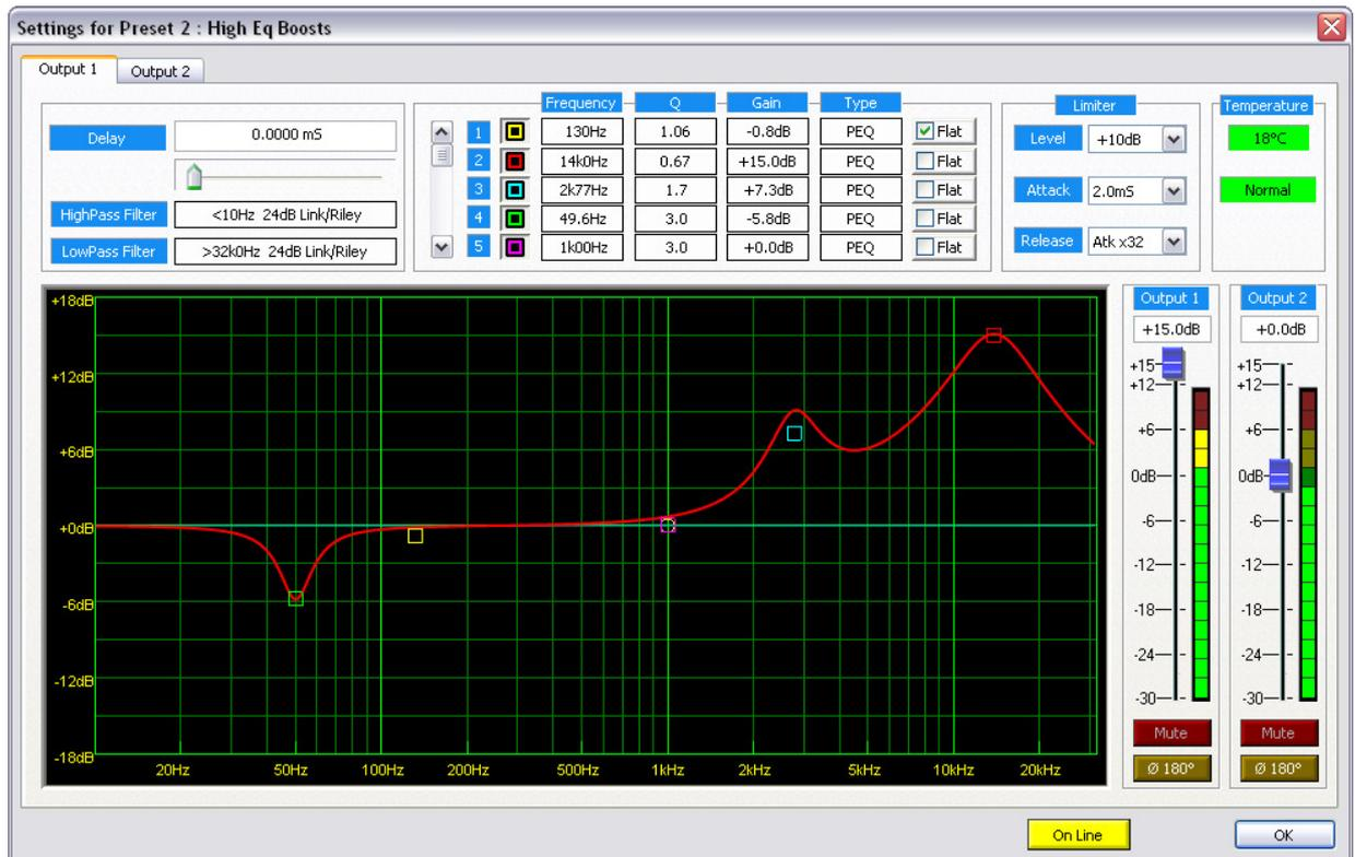
The tabs at the top of this screen select each output, with the gains, phase and mutes being available on both tabs all the time, along with the metering. All the DSP parameters are accessible on these two tabs, including the output delays, limiters, and gains.
