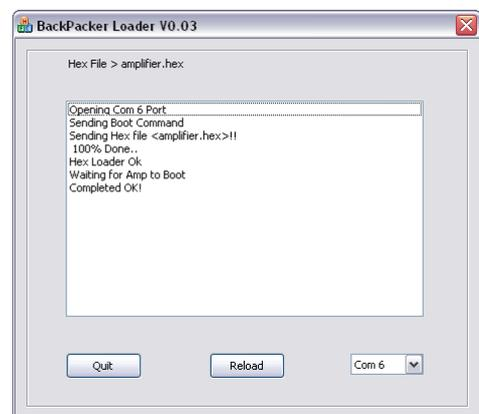
It is also possible to write a batch file to load new firmware AND a new preset file into an amplifier as a single procedure: this is explained overleaf...
