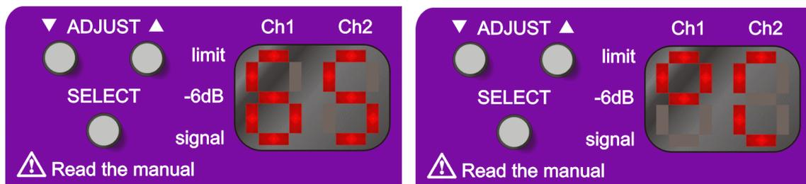
The temperature may continue to rise, and the amplifier will carry on working normally. Once the temperature reaches a level that is likely to cause damage to internal components, the amplifier will shut down, and display a flashing warning of the form below. (Warning code shown is for fan failure – E1 or E2 denote over temperature warnings).
