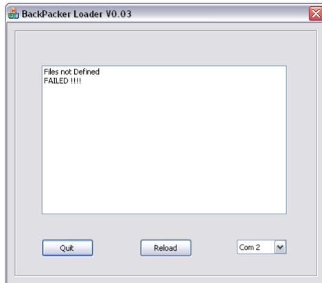
The program called BackPackLoad.exe will not, on its own automatically load any software or preset files. If you double click on the program to run it, it will display the message as shown.
