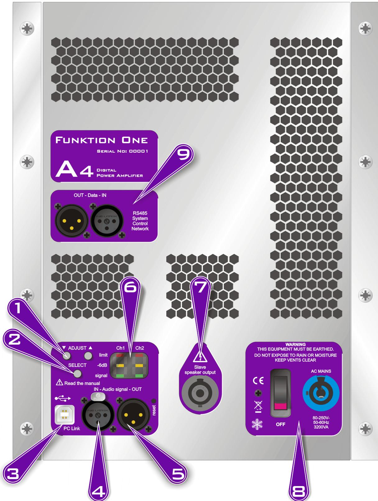
The diagram on the facing page shows all the external controls and connectors on the amplifier module. For information about the internal speaker connector, please see the appendices.
