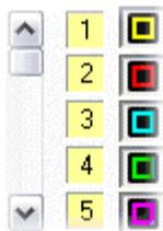
The set of buttons showing the filter markers for the curve view may be toggled on or off – this does not bypass the filter (its contribution to the overall response remains part of the curve) – it merely stops it being editable via curve dragging.
