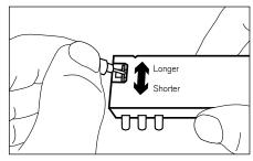
Using the screwdriver part of the adjustment tool, turn the rotaries in the directions shown to adjust the lag time.
