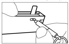
Please adjust with caution as the grub screw can be lost if unscrewed too far. (However a replacement can be found inside the top of the Torque Adjustment Tool.)
