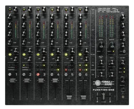
Channels 1 and 2 are switchable between microphone or stereo line inputs. These channels also both have a selectable compressor built in for further control. Channels 3 to 6 are switchable between stereo phono or line inputs. These channels have separate cross-fader routing selection. The contour of the cross-fader is adjustable to preference.
