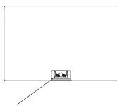
Recessed connector pockets for safety of cables and connectors
