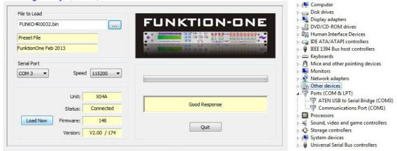
Set the Serial port in Funktion One Flash Loader to this number, and click connect. You should now be connected to the XO unit. Now at the top of the application window, click on the button next to "File To Load", navigate to your preset BIN file and double click on it or click Open. Now click the "Load Now" button. A popup will open to ask "Confirm Load Presets?" Click "OK"
