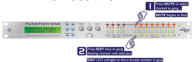
Press a **MUTE** key to choose the output to gang – its LED will begin to flash, and an **EDIT** key will illuminate to show which output it is currently ganged with. To change this selection, just press another **EDIT** key, remembering that gangs work from the highest to lowest number. So, to gang outputs 1 and 5, press **MUTE 5** then **EDIT 1** – the display will show
